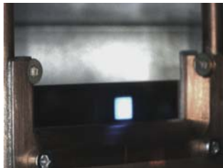
Fig. 1: First white beam light at the fluorescent screen 4 closest to the experiment deflected by all four mirrors.
