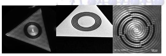
Using Archimedean spirals with broken n-fold radial symmetry, it is possible to excite surface plasmons with angular orbital momentum on the gold flakes (see right image). This leads in case of 4-fold symmetry to cloverleaf-type nanofoci on the order of 100 nm, which rotate during four optical cycles by 360 degrees.
