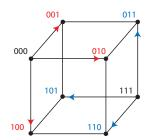
Note that the messages and their corresponding corrupted versions do not overlap, i.e. the 000 with corrupted version 001, 010, 10 does not overlap with 111 or 110, 101, 011. Thus it is possible to "undo" the effect of the noise by resetting the bits to the one obtain by taking a majority vote of the 3 bits at end. This resets 000, 001, 010, 100 to 000 and 111, 110, 101, 011 to 111. If we include the errors which occur to order  $p^2$ , we would not be able to correct them.
