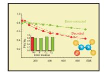
The demonstration of quantum error correction is in the shape of the green curve which does not have the first order error, i.e. with no error correcting (red curve) the fidelity goes as  $e^{-t/T_2} \approx 1 - t/T_2$  and if we have error correction as  $\approx 1 - c(t/T_2)^2 + \ldots$  The green curve is much flatter than the red one.
